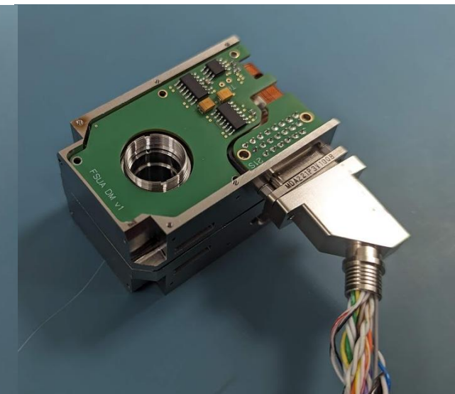
Czech contribution: Fibre Switch Unit Actuator (demonstration model) – will allow to switch between two laser beams
