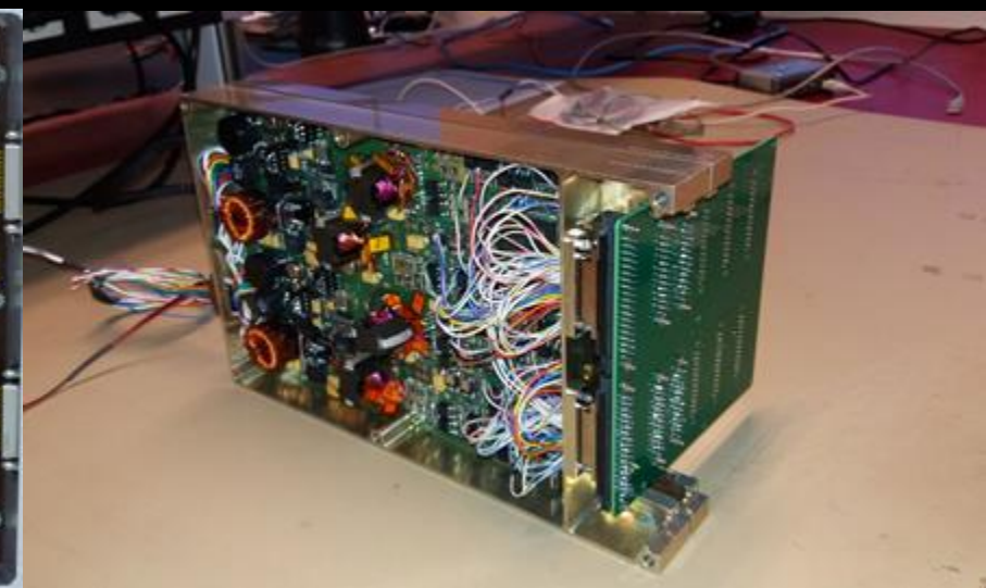
Low-Voltage Power Supply
